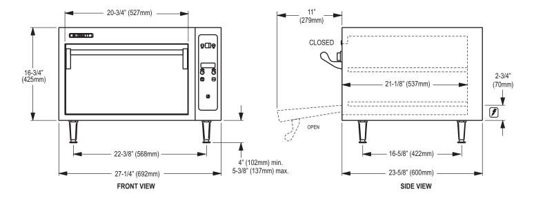
DIMENSIONS:SingleDoubleNumber of sections:12Number of controls:12Number of compartments:12
