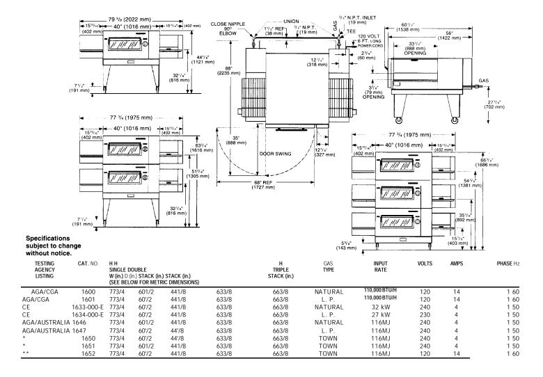
Metric Dimensions for all models: Width: 1975 mm; Depth: 1538 mm; Height Single Stack: 1121 mm; Height Double Stack: 1610 mm, Height Triple Stack: 1686 mm
