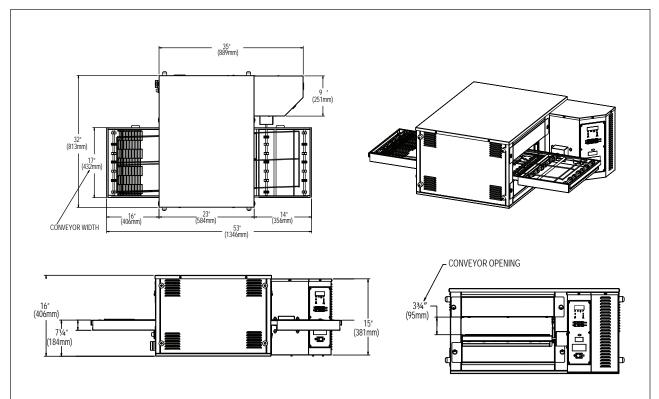
**ELECTRICAL SERVICE:** Heat is supplied by six (6) infrared elements at 1200W each, (user may select any three (3) elements to be activated at one time,) one (1) main fan element at 8000W. Each finisher is rated at 12 kW. The DTF-16 is available in 208V or 240V, 3-phase power. A separate circuit breaker is required for each finisher with the proper voltage, amperage, phase and hertz as indicated by model number. UNIT REQUIRES 50 AMP SERVICE. Plug type NEMA-15-50P.
