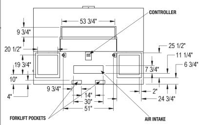
Optional storage boxes shown. Standard access panels correspond to outer dimensions of the storage boxes. All storage boxes and/or access panels must remain easily removable after installation.
