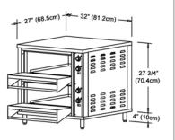
240v /1 phase 30 AMPS \*\*\* 208v /1 phase 35 AMPS \*\*\* 208v /3 phase 20 AMPS
